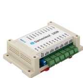
Damocles2 1208 12× DI, 8× DO OC, stand-alone device
