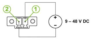
Figure 2: Connection of Power Supply
