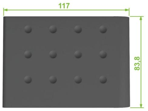
Figure 4: Plastic box – Top View
