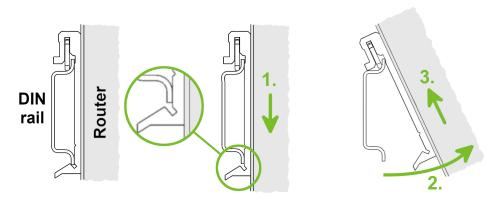
Figure 6: Removing Router from the DIN Rail
