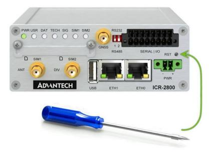
Figure 20: Resetting the Router
