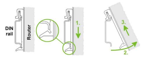
Figure 9: Removing Router from the DIN Rail
