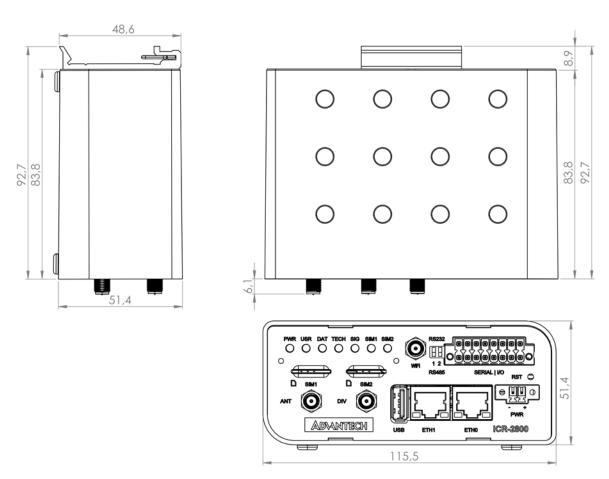
Figure 7: Plastic Box - Top, Side and Front View
