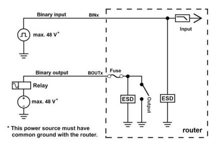
Figure 16: Functional Scheme of the Binary Interface
