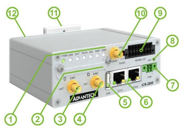
Figure 5: Hardware Overview of the Router
