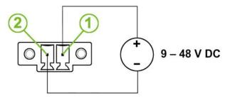
Figure 13: Connection of Power Supply
