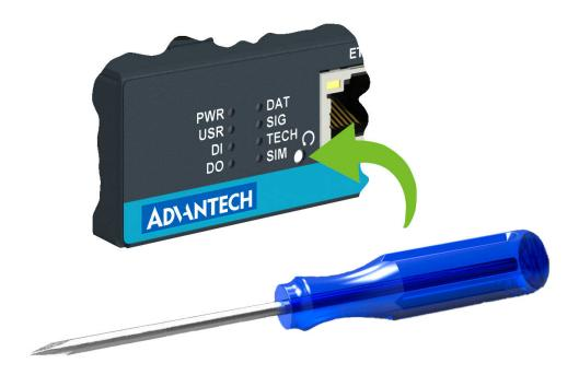
Figure 12: Resetting the Router
