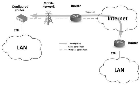
Figure 3: Using VPN Tunnel
