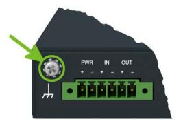
Figure 8: Position of the Grounding Screw
