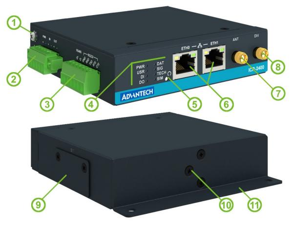
Figure 5: Hardware Overview of the Router
