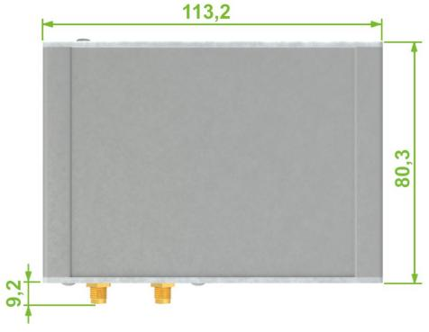
Figure 6: Metal box - Top View
