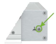
Figure 8: Position of the Grounding Screw
