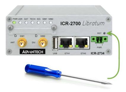
Figure 10: Resetting the Router
