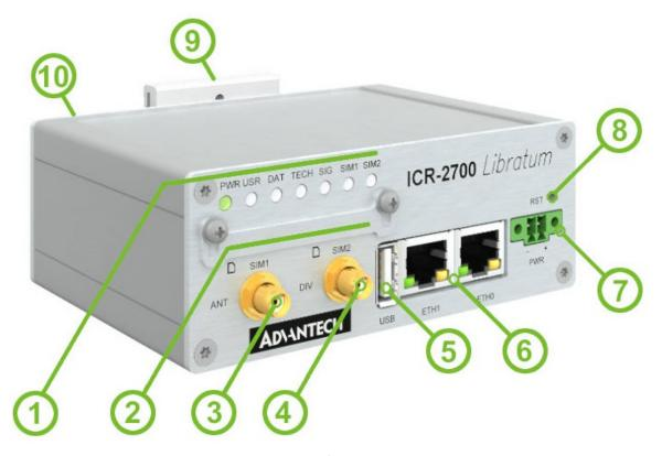
Figure 5: Hardware Overview of the Router
