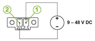
Figure 7: Connection of Power Supply
