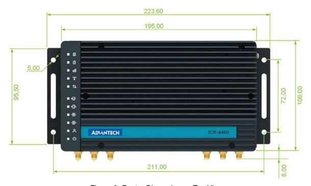
Figure 6: Router Dimensions - Top View
