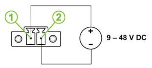
Figure 8: Power Connector Pinout
