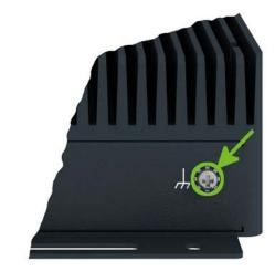
Figure 9: Position of the Grounding Screw
