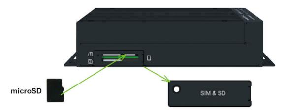
Figure 14: MicroSD Card Insertion
