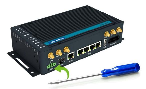
Figure 15: Resetting the Router
