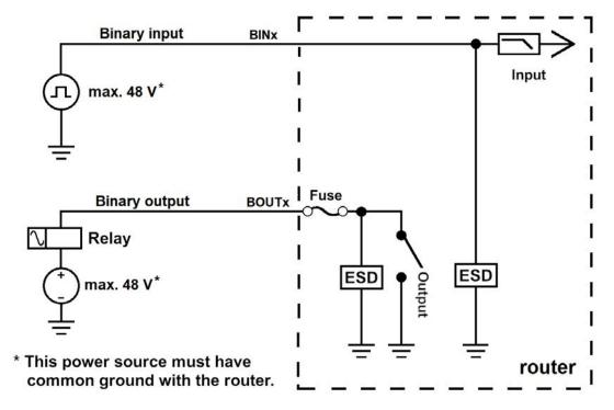
Figure 11: Functional Scheme of the Binary Interface
