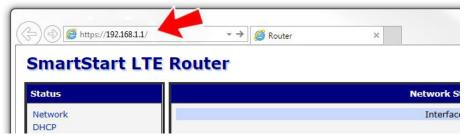
Figure 25: Entering the IP address of the router
