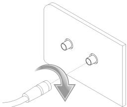
Figure 18: Connecting the antenna
