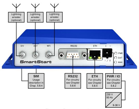
Figure 24: Router connection
