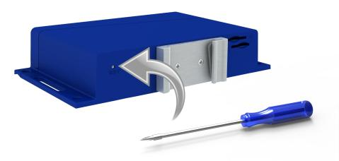
Figure 23: Router reset
