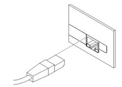
Figure 21: Connection of Ethernet cable
