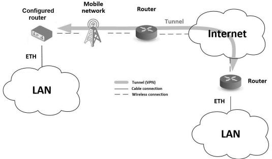
Figure 3: Using a VPN tunnel
