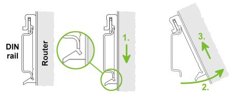
Figure 13: Removal from the DIN rail
