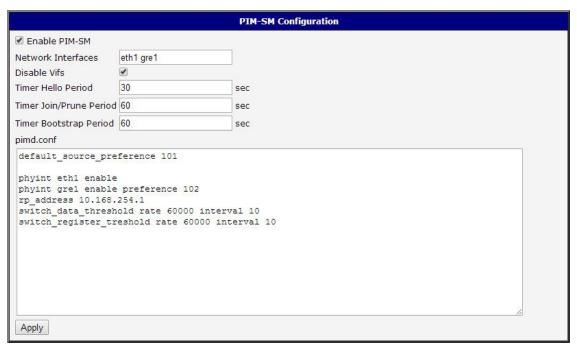
Figure 1: Static selection of RP
